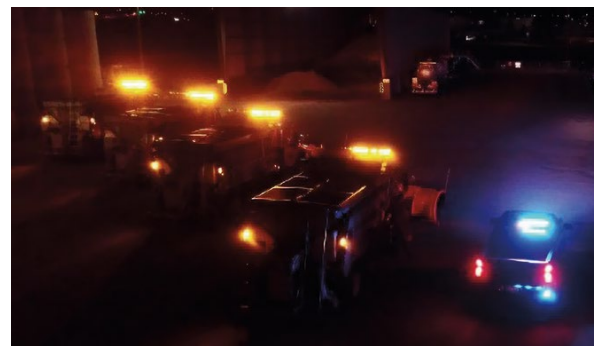
Figure 5-15: Example of synchronized emergency vehicle lighting. Source: Colorado Department of Transportation; Federal Highway Administration
