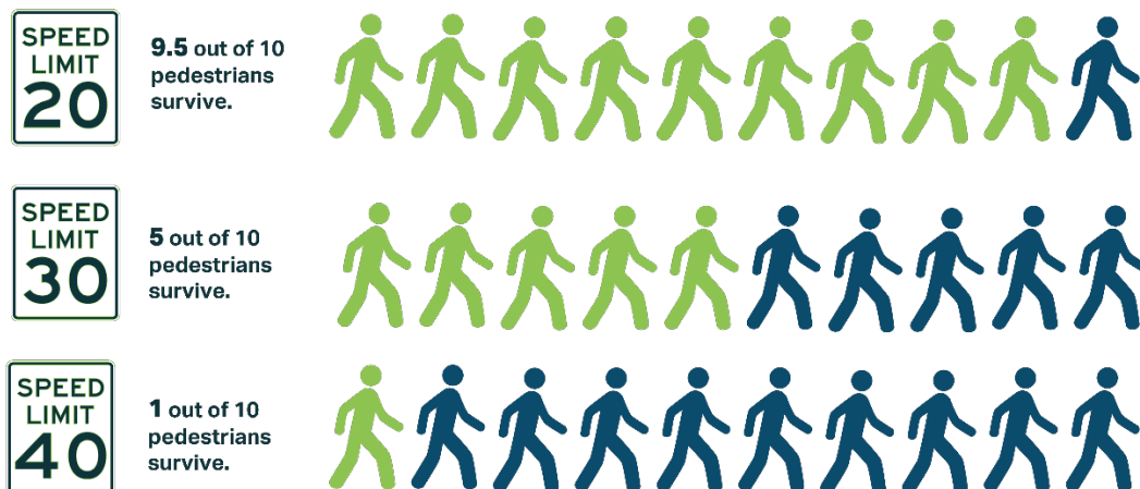
Figure 4-4: Pedestrian Crash Survival Probability at Various Vehicular Speeds (Source: NACTO Urban Street Design Guide)
