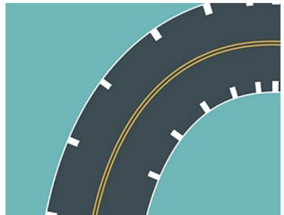
Figure 5-13: Optical Speed Bar Representation, Federal Highway Administration
