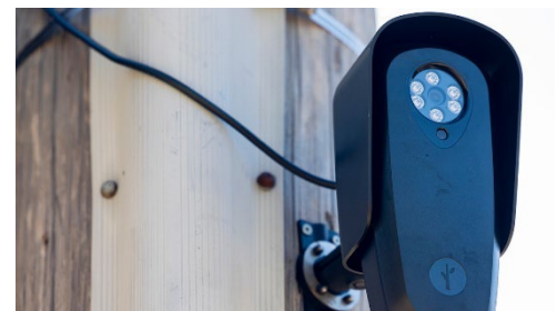
Figure 5-14: A Flock license plate reader camera used at intersections. Source: MLive Joel Bissel
