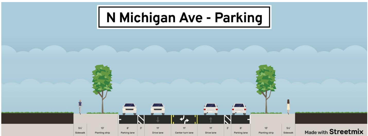
Figure 6-18: Alternative Cross Section 1A - Road Diet and On-Street Parking
